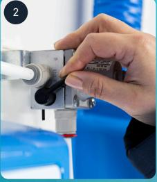
Turn off gas feeding empty keg. Remove keg coupler from empty keg and reconnect to new keg.
